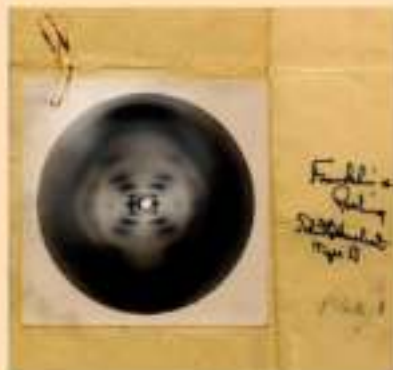
Photo 51 , taken by Franklin, is a 1952 X-ray diffraction image of human DNA. The X-shape is due to DNA's double-helix structure.
