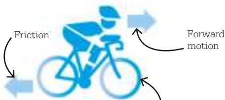
Bicycle in motion due to force supplied by rider's pedaling being greater than friction and drag (air resistance)
