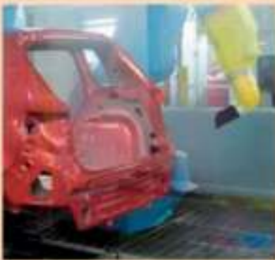
Paint robots at this Volkswagen factory help reduce employee costs, and can be programmed to use the minimum amount of paint required.
